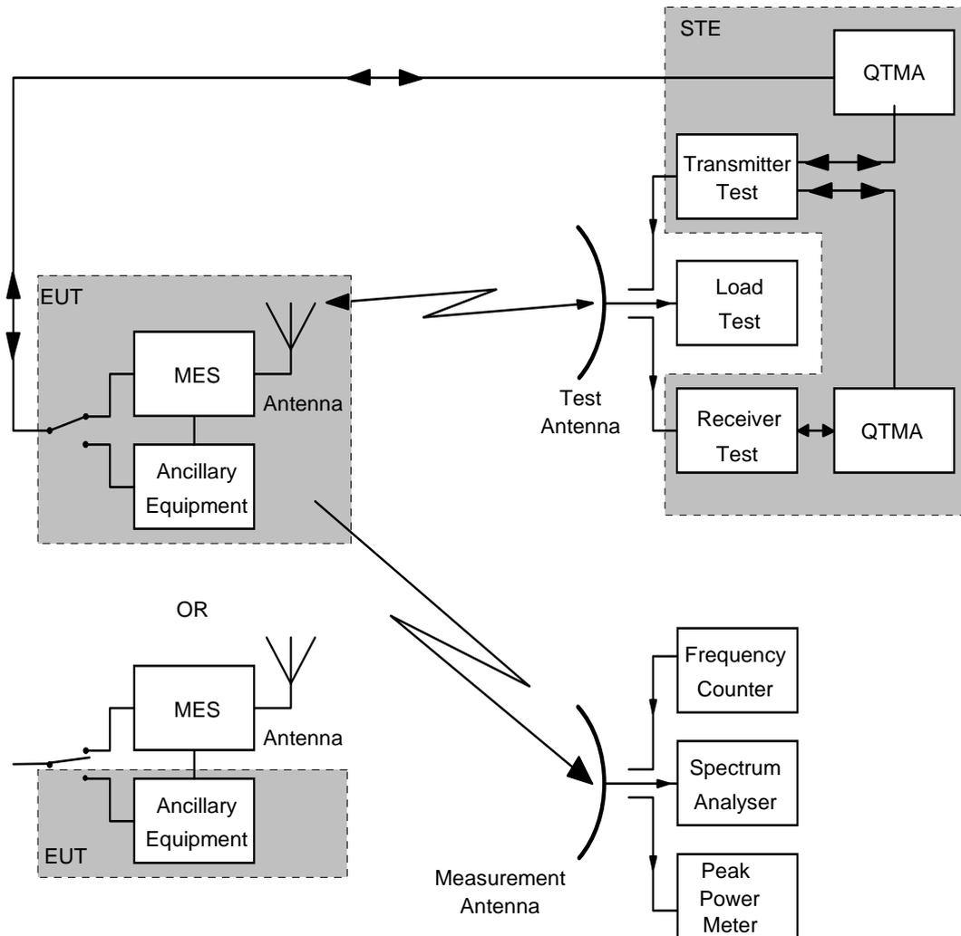
**Figure 1: Suggested test configuration**
